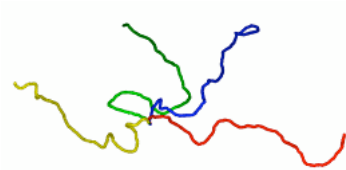
Fig. 5 Five examples of cellulose molecules obtained from computer simulations of cellobiose in water. From complete sets of such conformations physical properties like the persistence length are calculated.
